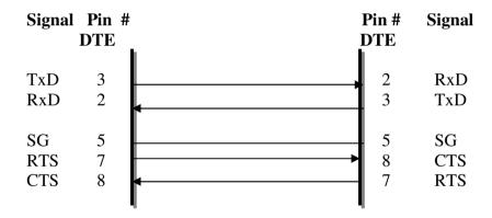
For loop back test, you can connect TxD(pin 3) to RxD(pin 2) and RTS(7) to CTS(8).
